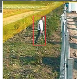
With a modern 3D-video sensor fences up to 50 m can be observed with one camera.
